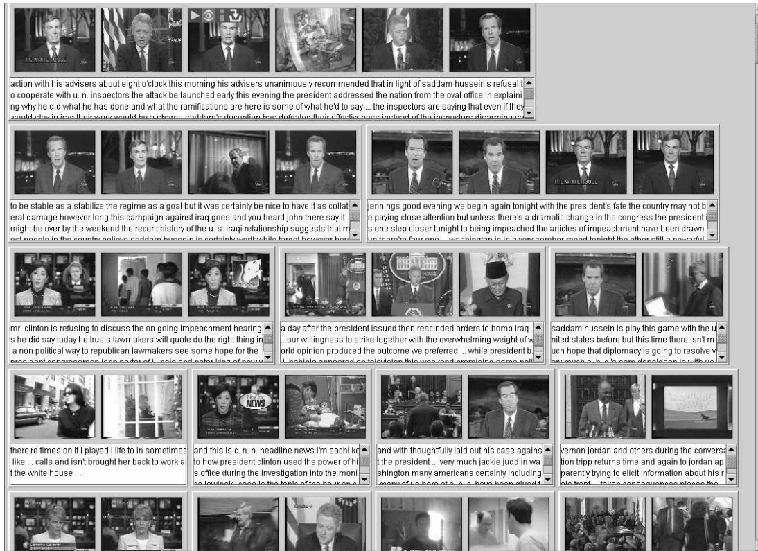
Figure 2. Alternative similarity view: shots are grouped together if they originate from the same video file. The results are displayed using shot key frames. Speech transcripts are visible under the key frame groups.
