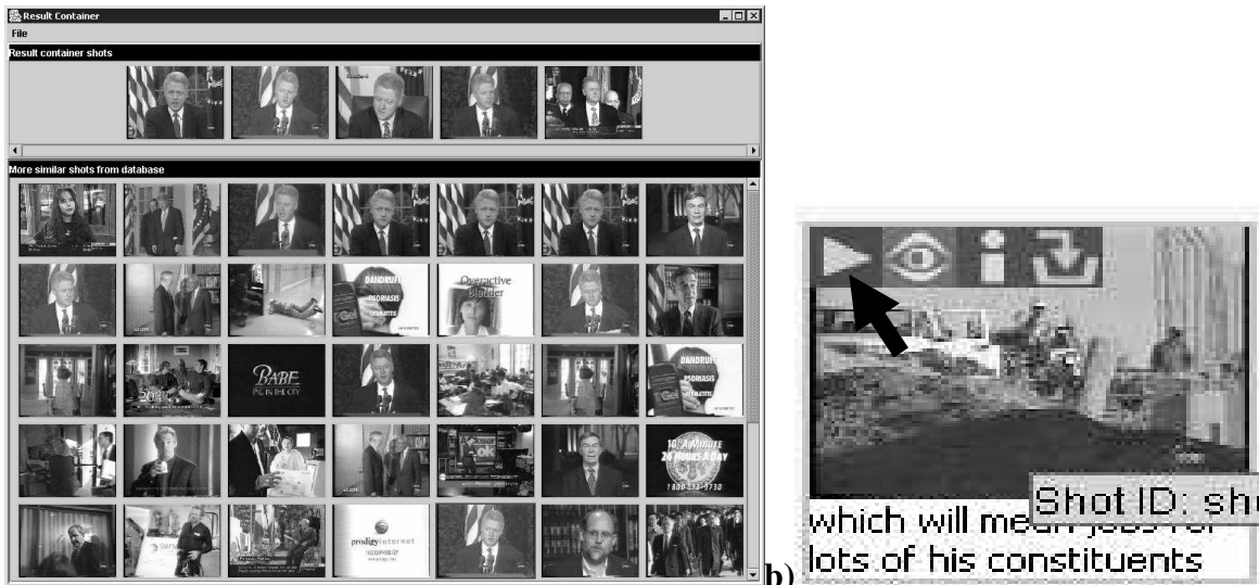
Figure 3. (a) Result container stores all the selected relevant shots and suggests more of similar shots based on the selected ones. (b) Fast action buttons are superimposed on each video item when mouse pointer is dragged over them.
