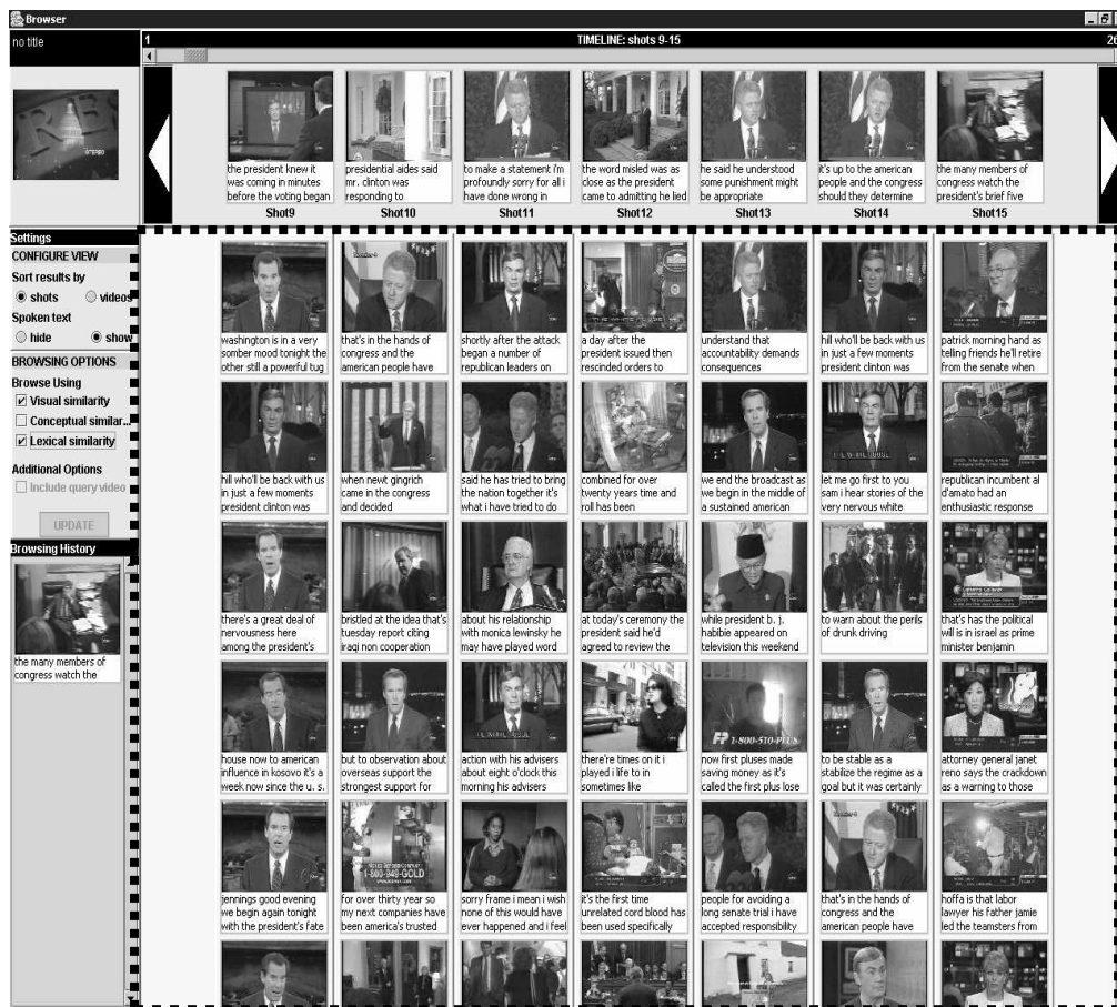
Figure 1. Cluster-temporal browsing interface. Dotted rectangle indicates the similarity view, where content-based result clusters are organized column-wise.
