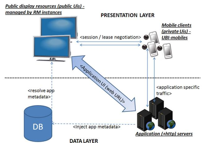
Figure 2. The distributed UI support in the OUSN. Mobile clients handle leasing of the displays and application servers provide the application’s public UI to the display resources.
